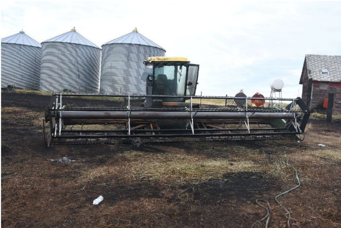
Figure 4 Photograph DSC_0015.JPG Front of John Deere 2420 Swather, Oxidation, Melting, Consumption, Charred Vegetation
