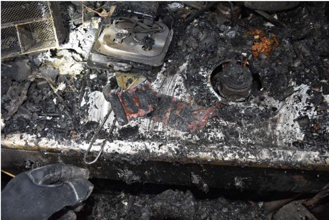
Figure 7 Photograph NJF_0069 Lithium-ion battery sheets discovered in kitchen
